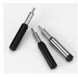
Pocket Penetrometers are commonly used on split spoon and thin walled tube samples to evaluate consistency and approximate unconfined compressive strength of saturated cohesive soils. They may also be used for the same purpose in freshly excavated trenches for the same purpose.
