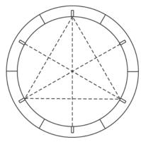
Reference points and anchors installed in pre-formed holes in concrete liner.
