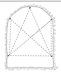
Reference points and anchors installed in drill holes in rock.
